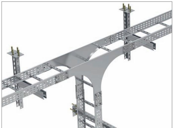
Vertical cable tray tees should be supported within 600 mm of each fitting extremity.
