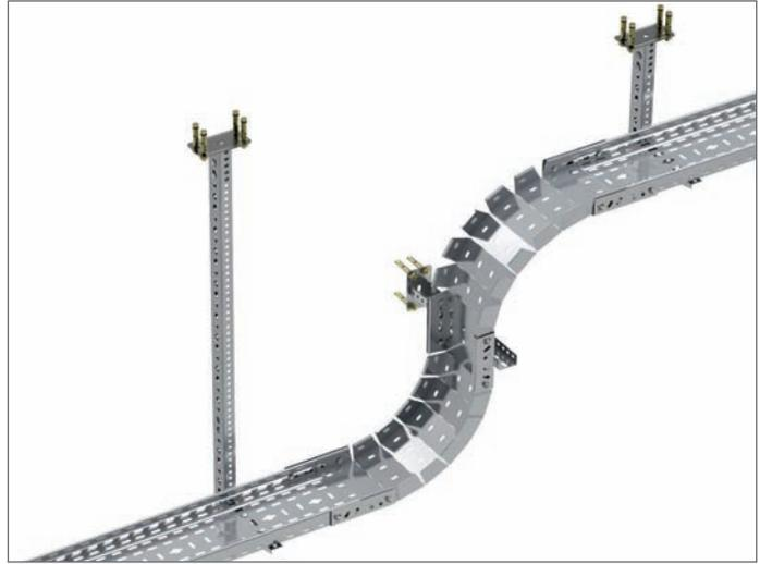
Vertical cable tray elbows at the top of runs should be supported at each end. At the bottom of runs, they should be supported at the top of the elbow and within 600 mm of the lower extremity of the elbows.
